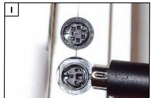
将血氧计连接到 9054 RPM-AutoAdjust
